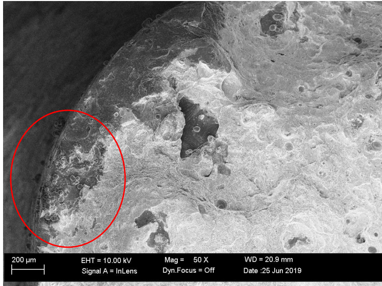
Figure 3.31 5 minute air cylinder #5 zoomed in fracture surface.
