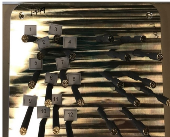
Figure 2.2 Completed build with number scheme used.
