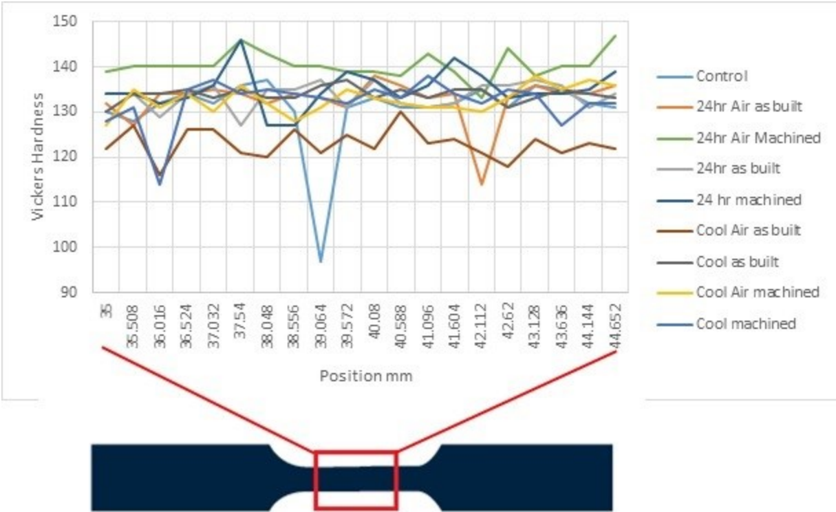
Figure 3.19 Vickers Microhardness measurements.
