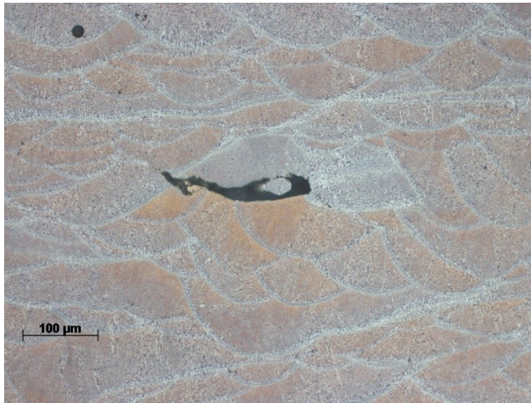
Figure 3.11 Complete cool air cylinder exposure showing a lack of fusion pore
