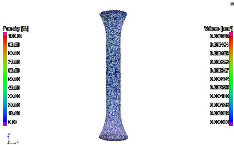
Figure 3.1 Control dog bone #5 with porosity and volume defect scale bars.
