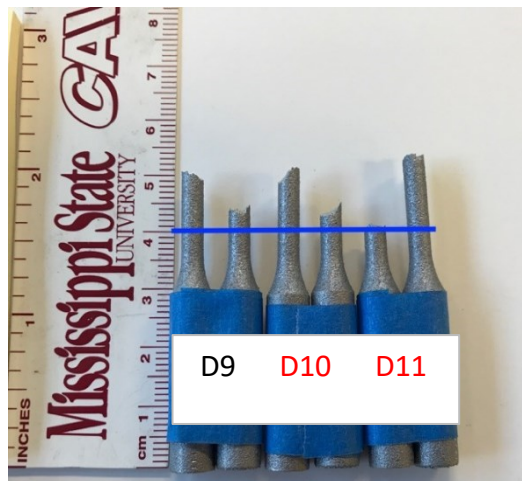
Figure B.30 24hr no air dog bone specimens
