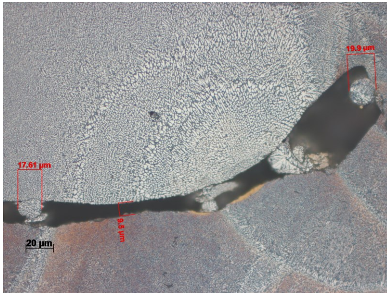
Figure 3.9 24 hour air cylinder lack of fusion pore
