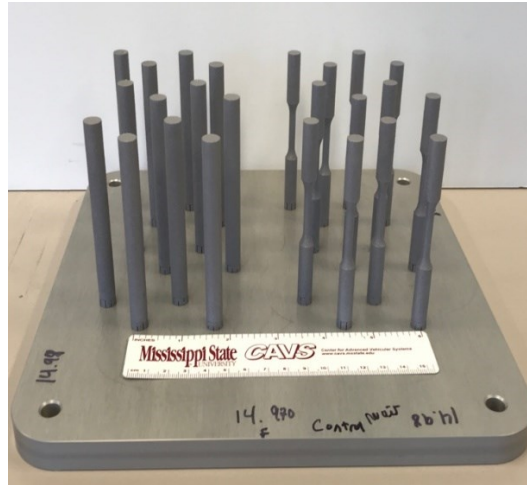
Figure 2.1 Completed control build showing layout of the specimens.
